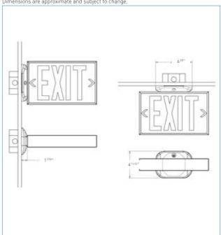
The  $\mathbf{EZ2^{\mathsf{TM}}}$  Canopy allows the installer to make all of the electrical connections using both hands without having to juggle with the Exit Sign, making it our most contractor friendly product feature to date. Simply attach the backplate to the junction box, clip the canopy on the Exit Sign, hang the canopy on the back plate, make your connections using both hands, slide the unit in place, one screw and the job is done!
