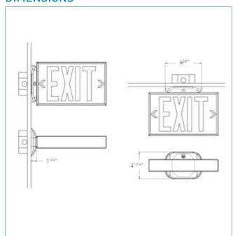
The EZ2™ Canopy allows the installer to make all of the electrical connections using both hands without having to juggle with the Exit Sign, making it our most contractor friendly product feature to date. Simply attach the backplate to the junction box, clip the canopy on the Exit Sign, hang the canopy on the back plate, make your connections using both hands, slide the unit in place, one screw and the job is done!
