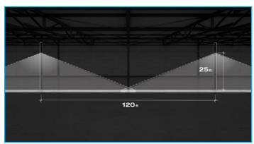
Installed at 25ft in the center of the space, the spacing is at 120ft
