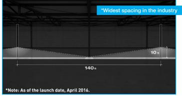
Installed at 10ft in the center of the space, the spacing is at 140ft
