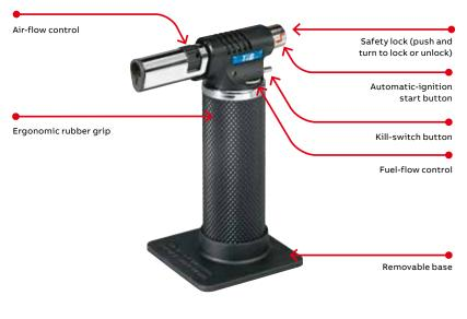
Portable heat shrink torch Separate fuel- and air-flow controls enable precise adjustment of flame and temperature to 1,371 °C (2,500 °F).
