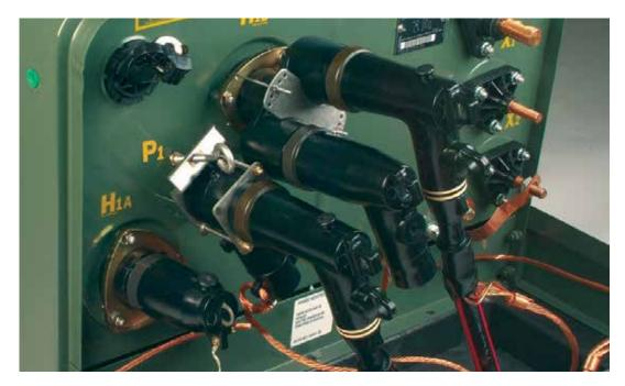
Conversion of a radial-feed transformer to a loop-feed, open-point transformer To convert a single-bushing transformer to a loop-feed, open-point transformer, add a parking stand arrester and an elbow arrester in combination with a feed-through insert.
