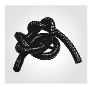
Extra flexible nonmetallic mechanical protection tubing is ideal for applications requiring extra strength and flexibility such as robotics and repetitive flexing arms. Carflex X-Flex is nonconductive, non-corrosive and resistant to oil, acid, ozone and alkaline. It's designed for use with standard Carflex fittings providing a complete nonmetallic system. Carflex X-Flex is lightweight for easier handling, transportation and installation.
