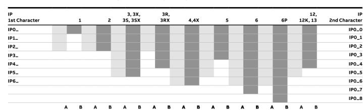
Conversion of NEMA enclosure type ratings to IEC 60529 enclosure Classification Designations (IP) (Cannot be used to convert Classification Designations to NEMA type ratings)
