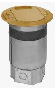
Recessed service, 3-gang pokethrough designed to fit in 6" holes in the second floor and above in commercial buildings. Given the limitations on the number of holes that can be drilled in a floor, it is important to maximize the capacity of each location. The RPT6 Series offers a configurable solution that provides high capacity for both power wiring and communications cabling—in a single-core drill location.
