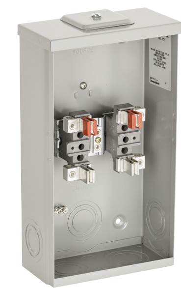
Microlectric® BE1-TCV Meter socket 100 A 600 V max 120/240 V single phase, 3 wires UNDERGROUND-ONLY APPLICATIONS
