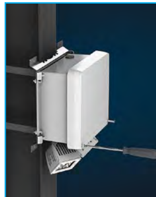
Unscrew access door screws.
